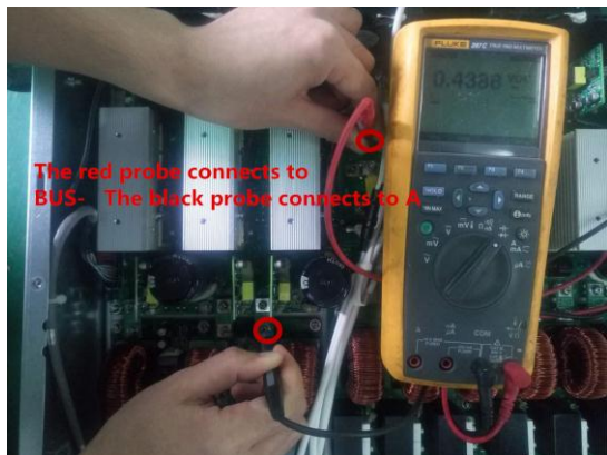
Fig.4-7 inverter IGBTs detect (b)
