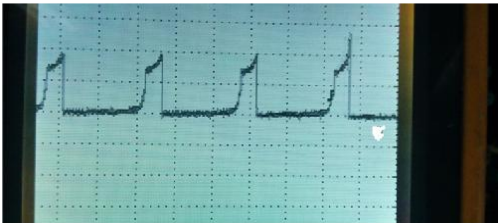
Figure 5.2 Drive signal of the SCR pin A-K
