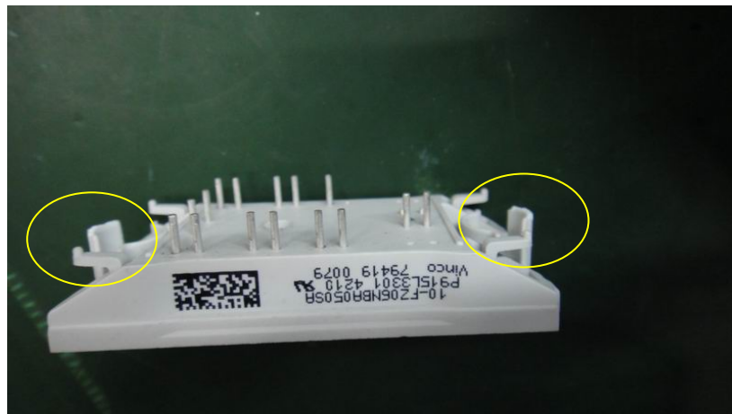
Cut off the fix nip of the new component before install it
