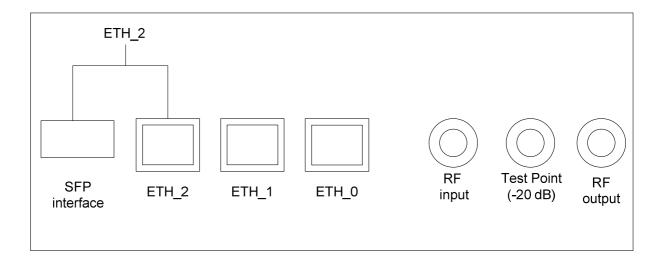
ETH\_2 is the preferred input port - if a connection is established (link-up), ROTON doesn't take into account any traffic from SFP interface. It happens only when ETH\_2 link is down and traffic connected to SFP interface.
