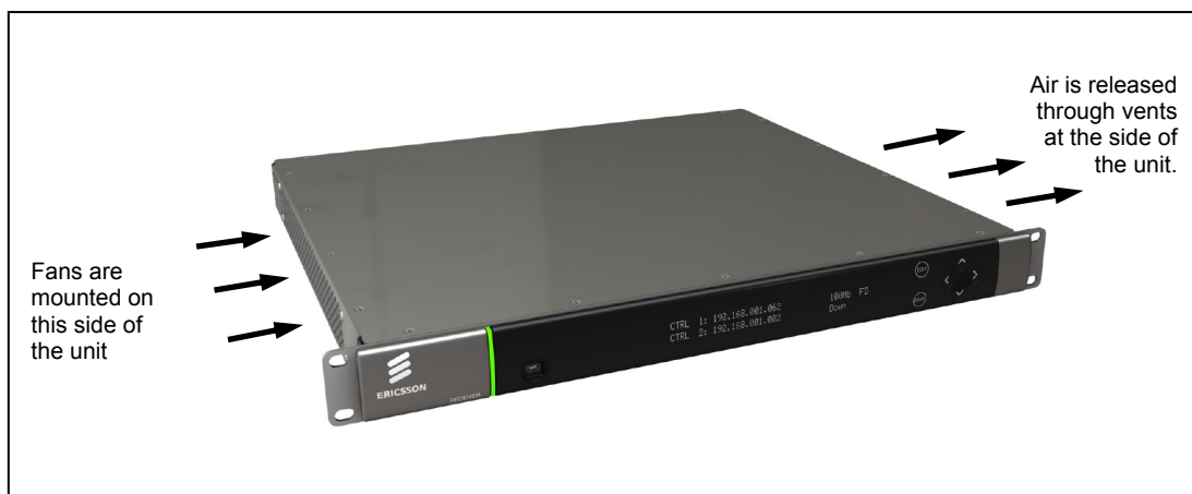
Figure 2.1 Air-Flow Through the Equipment
