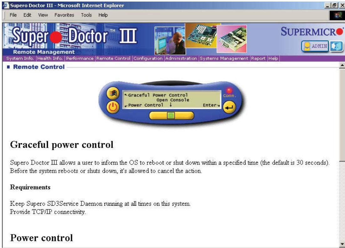
Figure 5-7. SuperDoctor III Interface Display Screen (Remote Control)
