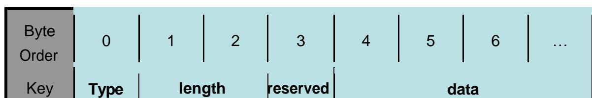
Extend header length must be multiple of 4 bytes;
