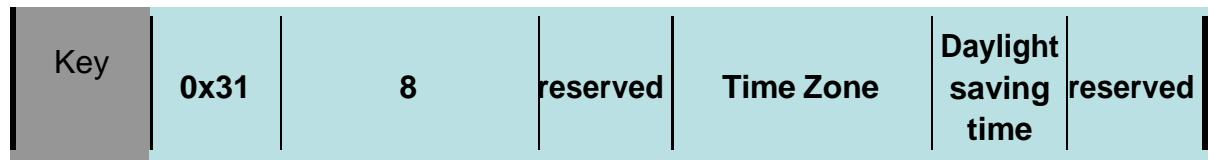
When a stream begin, or the TimeZone changes, the video packet must contain the TimeZone extend header; Time Zone[0]: [-12,12](west time zone 12 to east time zone 12), Time Zone[1] modify the time by minutes; Daylight saving time: 1/0, yes or not in daylight saving time;
