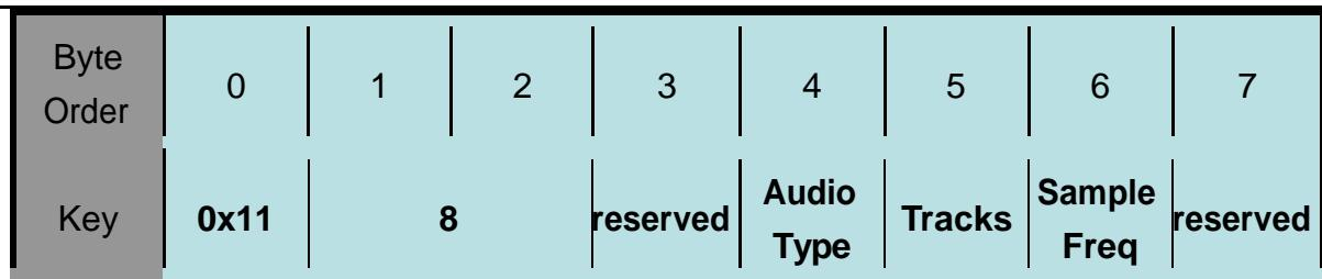
A audio packet must contain the audio extend header;
