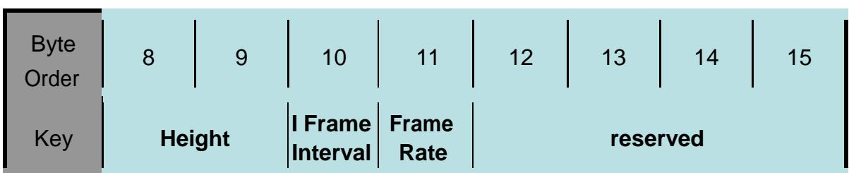
A video packet must contain the video extend header; Video Type means the video codec type, 1-MPEG4; 2-H.264; Frame Type: 1-I frame; 2-P frame;3-B frame; Width and Height describe the frame width and height by pixel;
