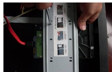
3. Use four screws to fix HDD.
