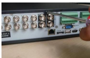
1. Loosen the screws of the upper cover.
