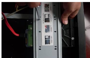
2. Line up the HDD to the four holes of the HDD bracket.
