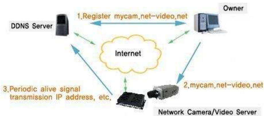
The DDNS process flow diagram of IP camera
