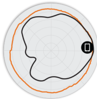
Figure 3. T310d 5GHz Azimuth Antenna Patterns
