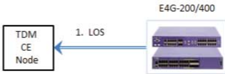
Figure 19: LOS Alarm Generation
