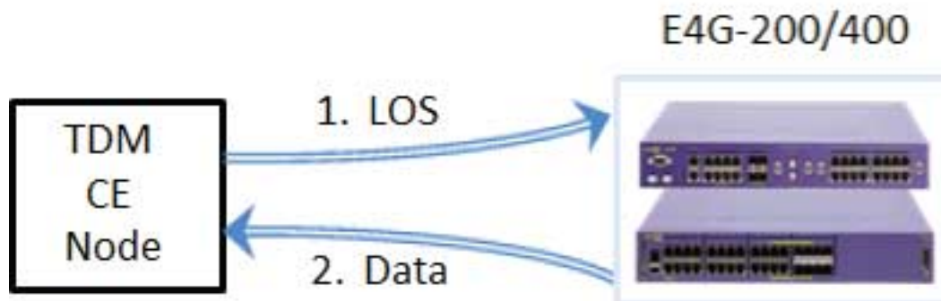
Figure 16: LOS Alarm Response
