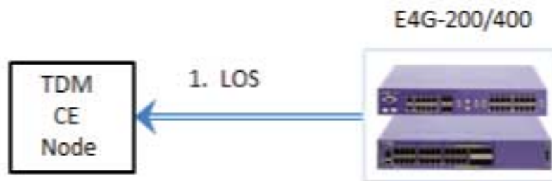
Figure 15: LOS Alarm Generation
