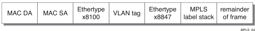
Figure 175: MPLS Unicast Frame on Tagged Ethernet VLAN
