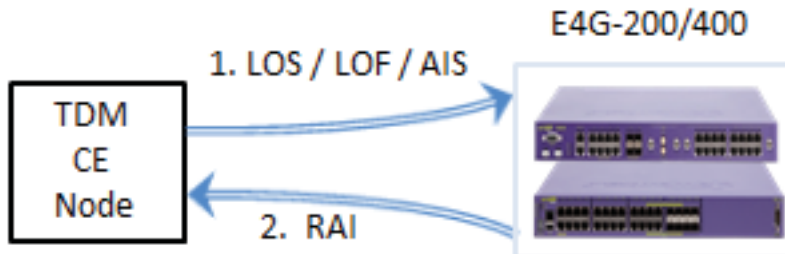
Figure 21: LOS/LOF/AIS Alarm Response
