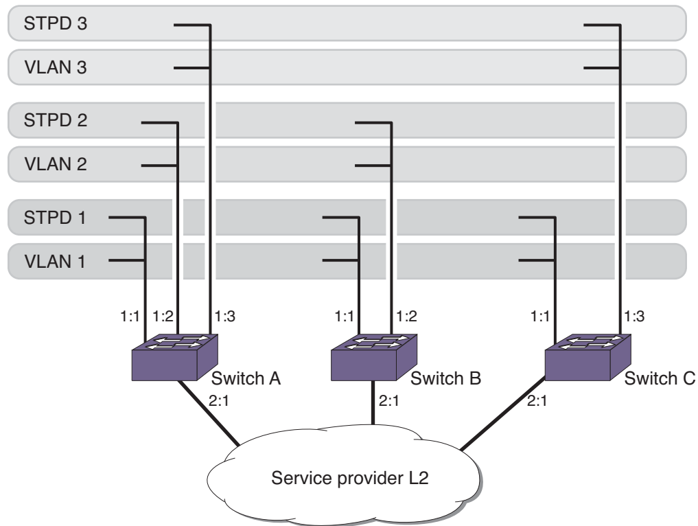
Figure 137: Sample Network Using STPD BPDU Tunneling
