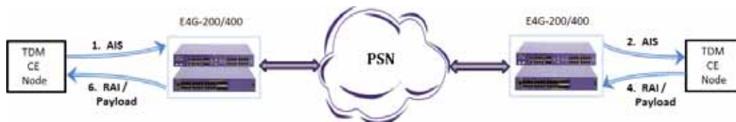
Figure 24: SAToP Alarm Handling: TDM Service AIS Alarm
