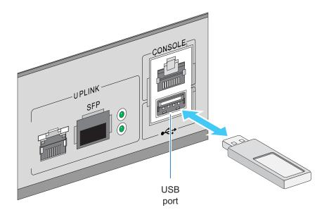
The Summit WM3400 wireless LAN controller contains one USB port for connecting USB flash storage devices to the controller. The controller can use the USB flash storage device for file transfers and firmware updates. Follow the setup instructions below to connect the devices to the controller and then access those devices through the Web UI or Command Line Interface.
