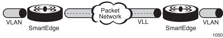
Figure 2 L2VPN Cross-Connection
