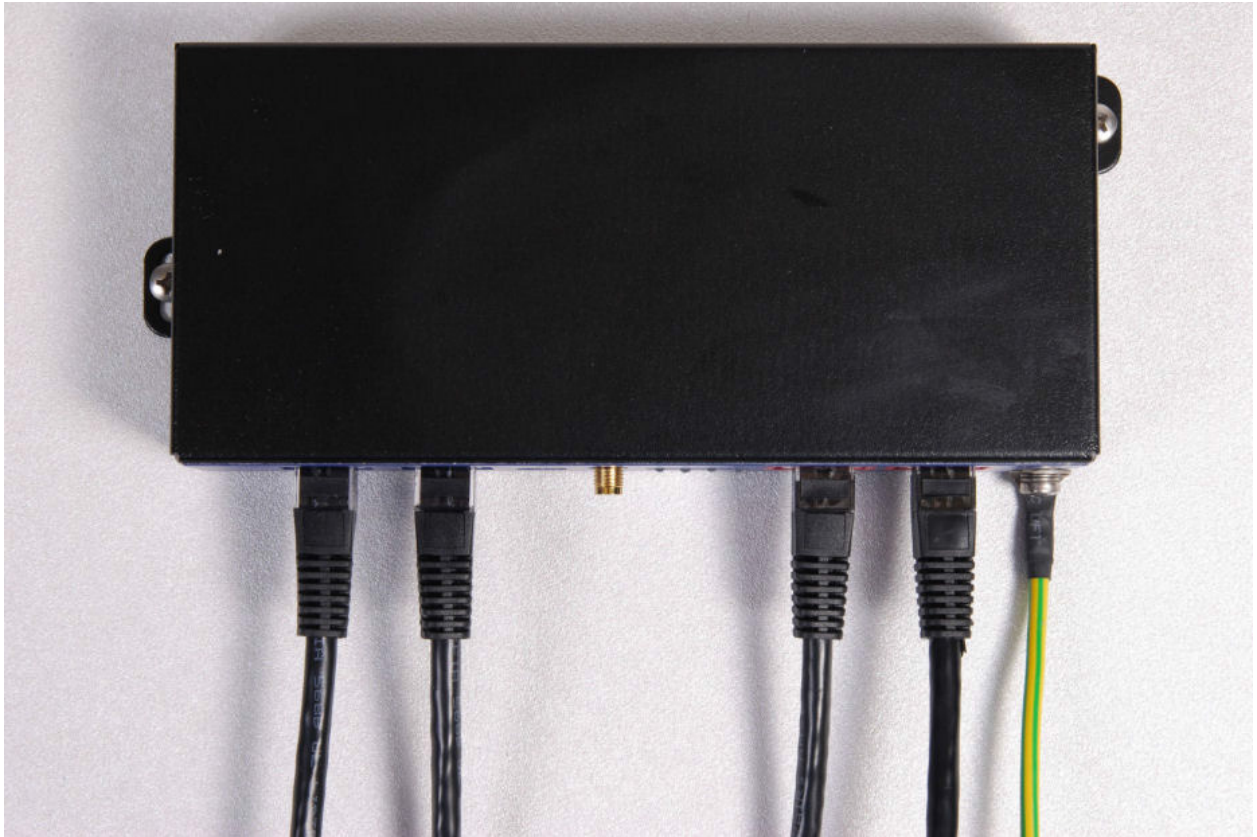
Figure 103 PTP-SYNC mounted on a wall
