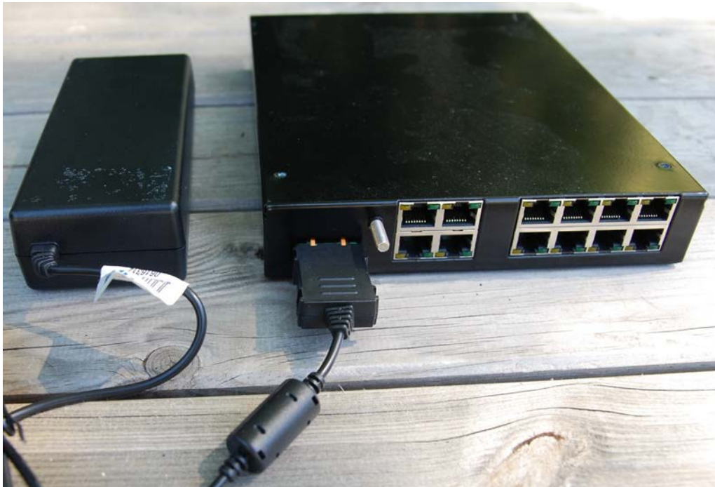
Figure 111 NIDU powered by the PTP 800 AC-DC Power Supply Converter
