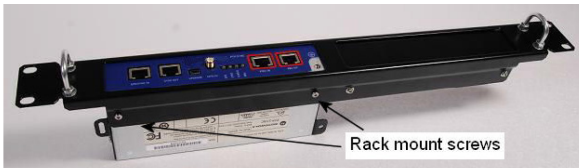
Figure 102 PTP-SYNC mounted in a rack
