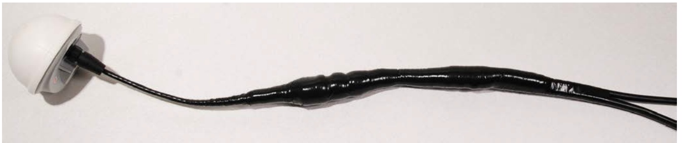
Figure 108 Grounding and weatherproofing example for GPS adapter cable
