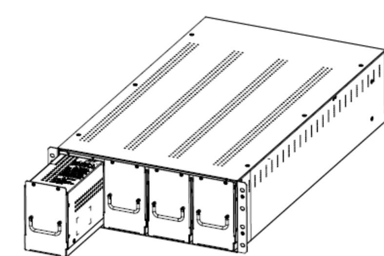
**Step 5:** put on the cabinet breaker. Use a multimeter to test whether the voltage of the battery cabinet port is normal. The positive voltage is greater than 240VDC, the negative voltage is greater than 240VDC, and the positive to negative voltage is greater than 480VDC.
