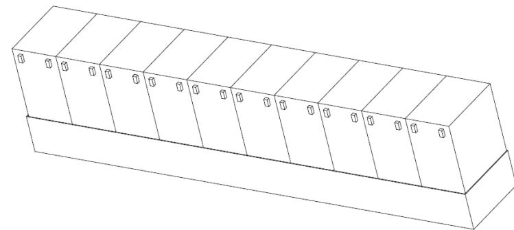
**Step 3:** push the battery and plastic pad into the battery pack from the front as shown in the picture below, connect the battery cable, and lock the front cover and top cover of the battery pack.
