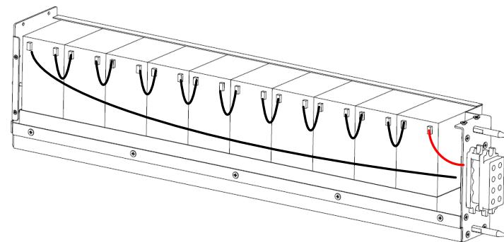
**Step 4:** test the voltage of the battery port to ensure it exceeds 120VDC, and insert the installed metal battery pack into the battery cabinet.
