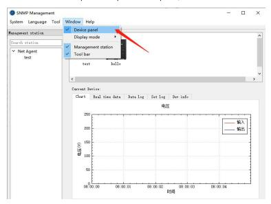
1) Chart: Display the dynamic curve diagram of the input and output voltage of the device, and can visually observe the changes of input and output voltage in real time.
