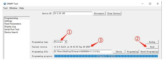
(3) Upgrade the application, ①Programming type select "APP" ②Select the new version file(file type is snmp-20xxxxxx-v1.x.x.xz.bin), ③Click "Programming", wait about 30 seconds, it will prompt "Programming finish".And then log in the background of SNMP card to check the software version.
