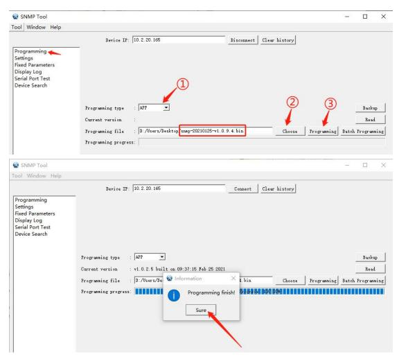
Check whether the application upgrade is successful, as shown in the figure below: Programming - Programming type "Select APP"- Read - check the current software version.
