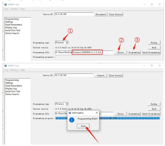
Check whether the firmware upgrade is successful, as shown in the figure below: Programming --Programming type--select "firmware"-- Read -- check the current program version.
