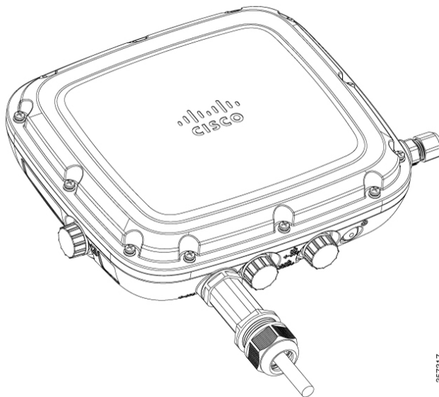
Figure 80: Fiber-Optic cable and gland installed to AP
