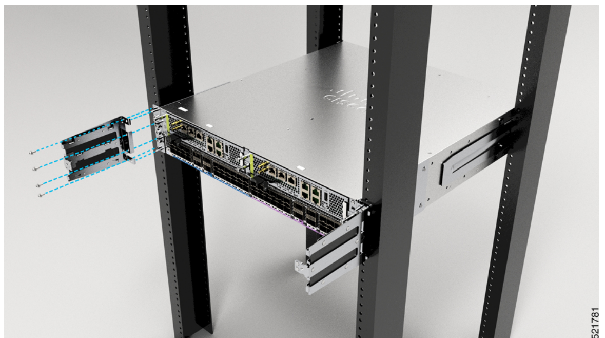
Figure 129: Cable-Management Bracket Installation and Removal-Cisco ASR 9902 Router
