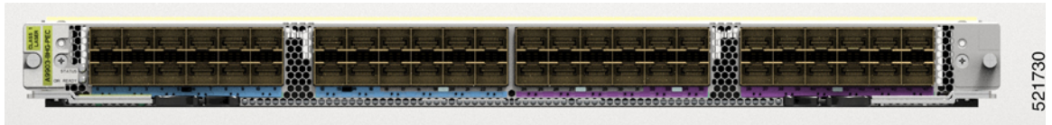
Figure 147: Cisco ASR 9903 Series 800G Port Expansion Card – Top View
